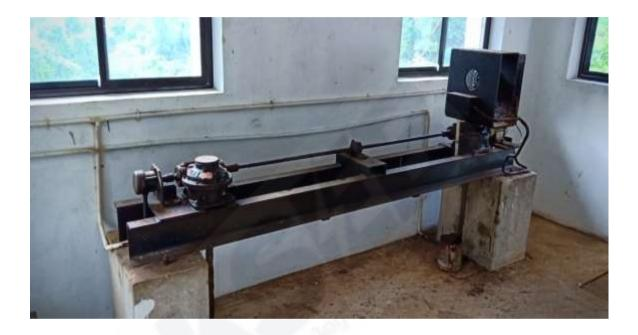
Fig 2.17 Operating gear of Disperser valve
